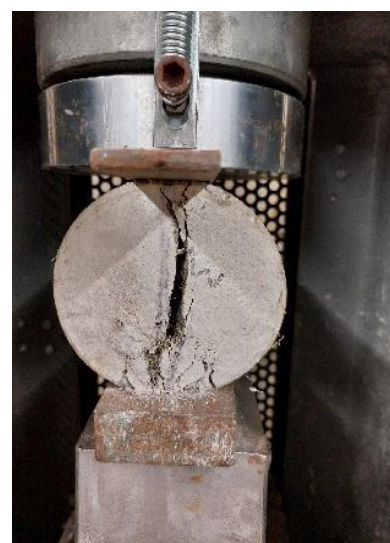
Figure 5. Split Sample from the Splitting Tensile Strength Test
