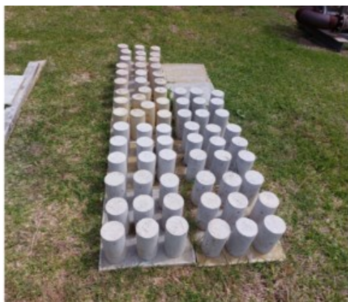
Figure 3. Array of Concrete Cylinders in Outside Exposure Condition
