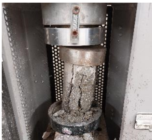
Figure 4. Crushed Sample from Compressive Strength Test
