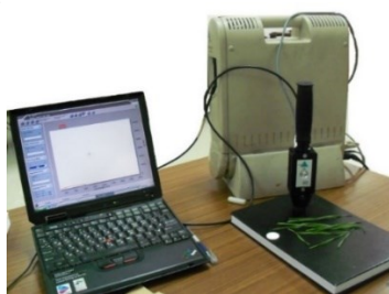
Figure 7. FieldSpec®Pro Device for Measuring Spectral Reflectance in the Field
