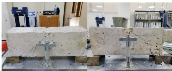
Figure 10. Control beam Cracks
