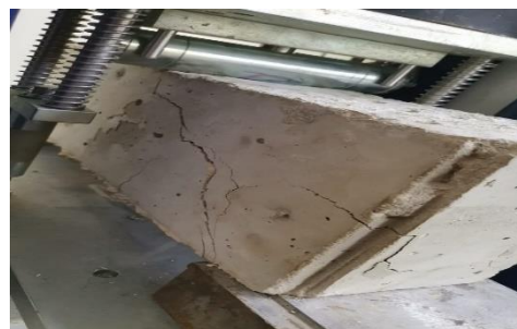
Figure 12. Beam B4 (U-section) Cracks
