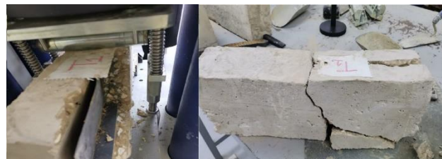
Figure 13. Beam B2 (inverted T-section) Cracks.
